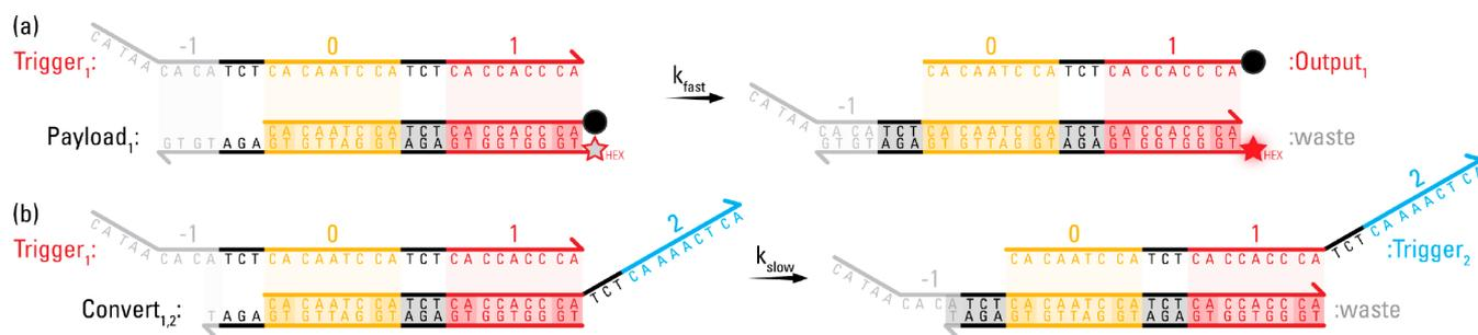
**Figure 2.** DNA strand-displacement (DSD) reactions for sequential release. (a) Example payload reaction in which a Trigger<sub>1</sub> strand releases an Output<sub>1</sub> strand from a Payload<sub>1</sub> complex. (b) Example convert reaction in which a Trigger<sub>1</sub> strand reacts with a Convert<sub>1,2</sub> complex to release a Trigger<sub>2</sub> strand.
