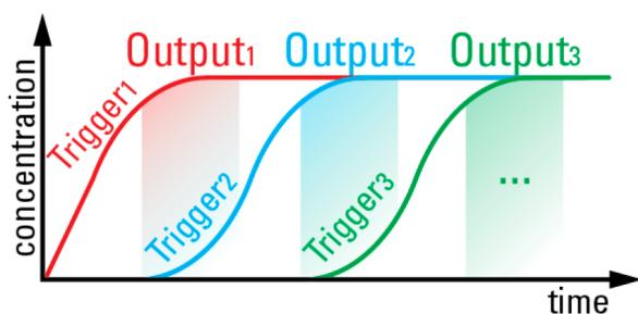
**Figure 1.** Sequential release. At each stage, an output molecule is released, after which the next output stage is triggered. In the schematic example, the completion of the red stage triggers the start of the cyan stage, and the completion of the cyan stage triggers the start of the green stage. Staged release could proceed over further stages.
