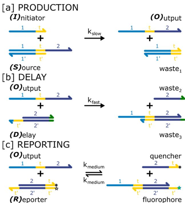
**Figure 2.** Strand-displacement reactions for a timer circuit. (a) PRODUCTION: Output is slowly released from source in the presence of initiator. (b) DELAY: Output is rapidly consumed by the delay complex. (c) REPORTING: Free output binds reversibly to a reporter complex, separating quencher and fluorophore modifiers. FAM and TexasRed paired with appropriate quenchers were used to report on two different output sequences (SI 0).
