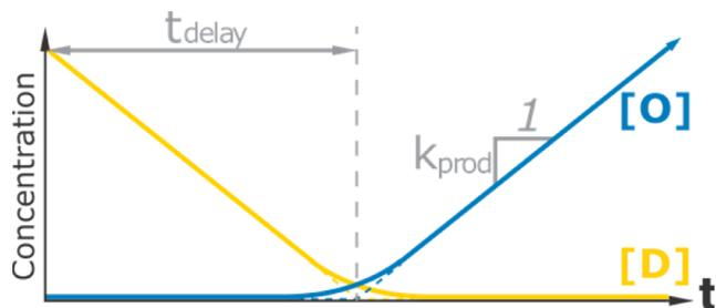
**Figure 1.** Schematic for the operation of a timer circuit. The output species (blue) is constantly produced at rate  $k_{\text{prod}}$  but is rapidly consumed by the delay species (yellow). This rapid consumption prevents the accumulation of output until time  $t_{\text{delay}}$ , when the delay species is depleted.
